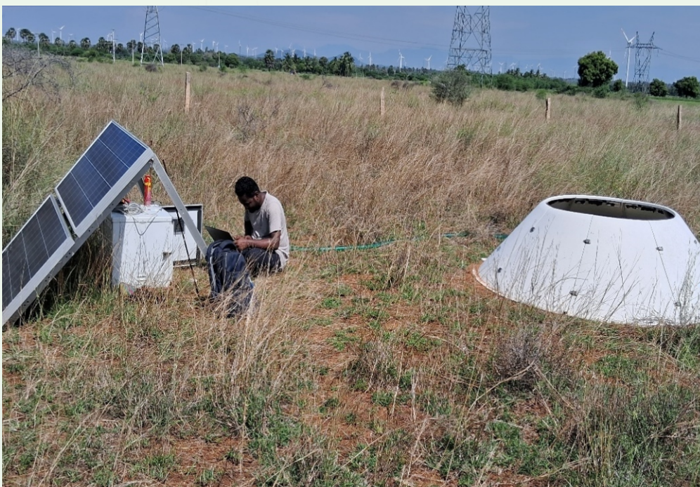
SoDAR Rectification work at Kayathar in progress
